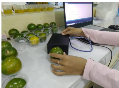
Figure 3. The reflectance measurement using handheld NIR spectrometer.
