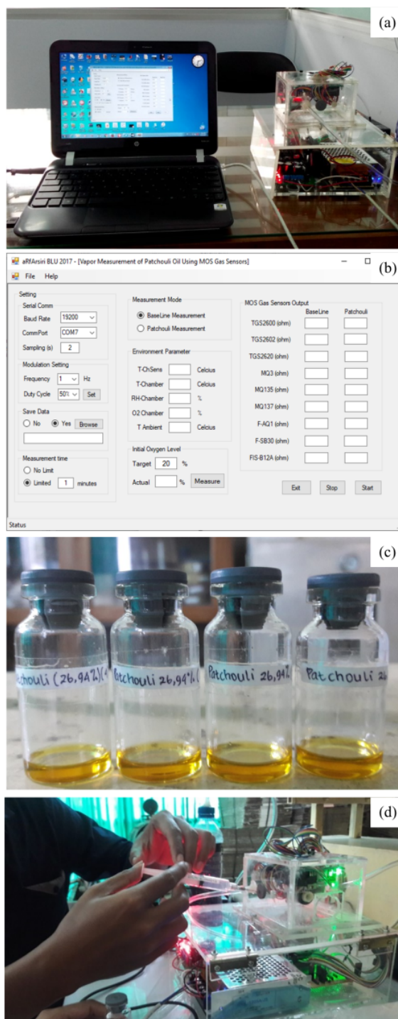
Figure 3. (a) measurement apparatus, (b) software interface, (c) static headspace vial, and (d) vapor injection process.
