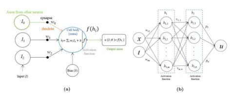
Figure 1. ANN Perceptron 1 (a) and multi-layered perceptron (MLP) 1 (b) architectures.
