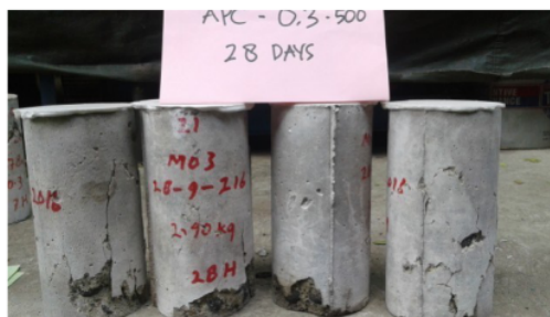
Fig. 10. Rupture of concrete cylinders containing coated plastic aggregate
