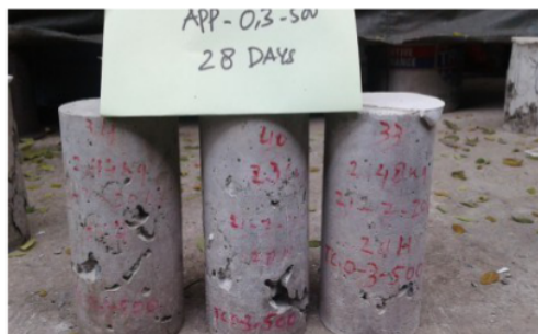
Fig. 9. Rupture of concrete cylinders containing uncoated plastic aggregate
