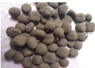
Fig.2. Plastic aggregate coated with sand
