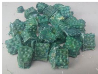
Fig.1. Shape of uncoated plastic aggregate [7]
