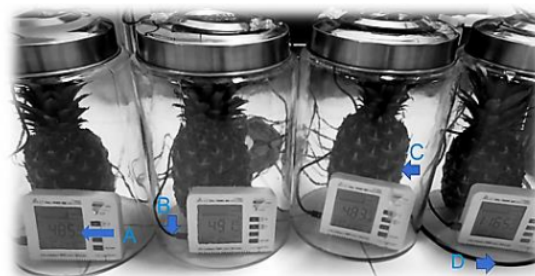
Figure 1. Experimental set up respiration rate measurement. A) CO 2 detector, B) Electricity cable of the detector introduced by the top, C) Pineapple fruit, and D) Sealed container.
