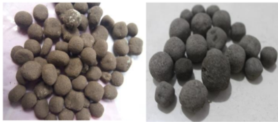
Figure 1 PP waste coarse aggregates: (a) coated plastic aggregate shape with river sand (RS), (b) coated plastic aggregate shape with volcanic sand (VS)
