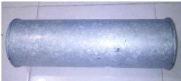
Figure 2. Muffler without re-heater.
