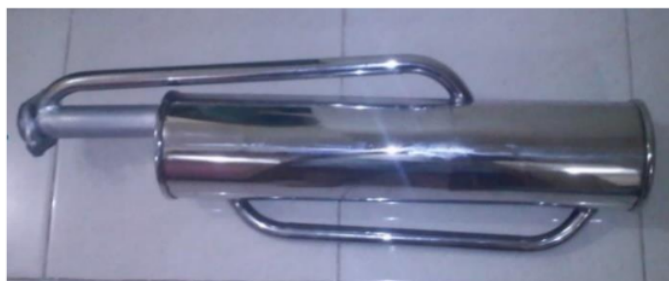
Figure 7. Real form of the muffler with re-heater.
