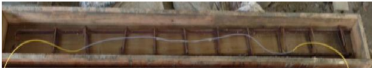
Figure 4. fiber optic configuration inside the concrete mold
