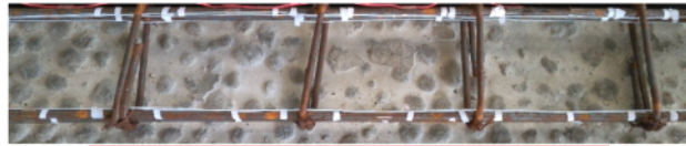
FIGURE 4 Fiber optic with straight configuration
