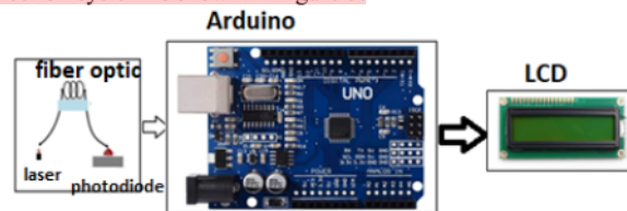
FIGURE 3. Block diagram failure detection system
