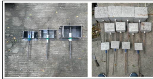
Fig. 2. Moulds and specimens for bond test
