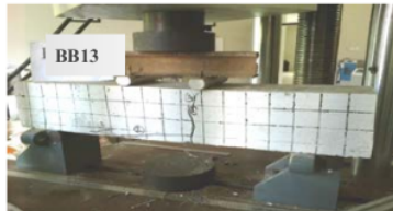
(b) Beam bamboo with mortar M13 (BB13)
