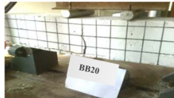
(c) Beam bamboo with mortar M20 (BB20)
