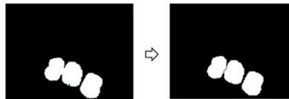
Figure 4. Separation of Objects Coinciding with Watershed Segmentation
