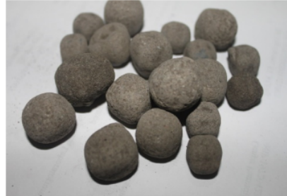
Fig. 3 Polypropylene waste coarse aggregate coated with sand
