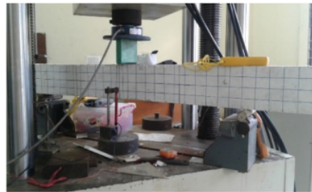
Fig. 6 Three-point bending test for RC beam
