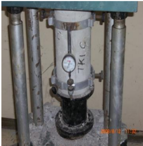
Figure 4. Compressive strength test [3, 18].
