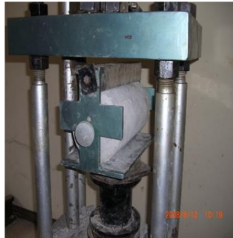
Figure 5. Split tensile strength test [3, 18].
