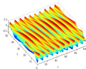
**Figure 4.** Signal of bi-chromatic wave at  $t = 120$  s for  $a = 0.1771$  m,  $k_{1x} = 1,2511$ /m,  $k_{1y} = 1,1617$ /m.
