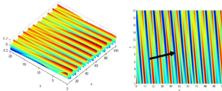
**Figure 2.** The bi-chromatic signal at  $t = 0$  (left) and the direction of wave propagation (right).
