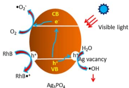
Fig. 8. The proposed mechanism of photocatalytic reaction in the surface of defect \text{Ag}_3\text{PO}_4 .
