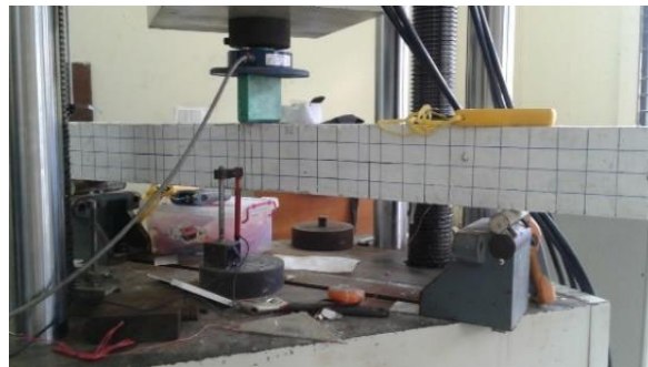
Fig. 6 Three-point bending test for RC beam
