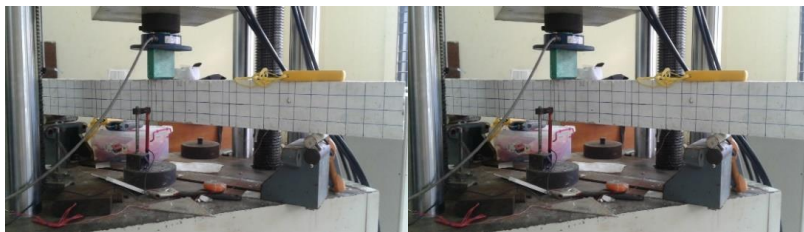
Fig. 6 Three points pending test for RC beam
