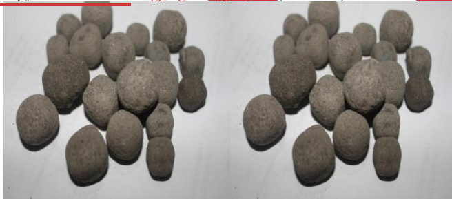
Fig. 3 Polypropylene waste coarse aggregate coated with sand
