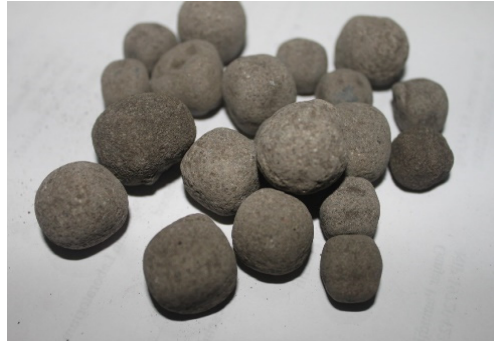
Fig. 3 Polypropylene waste coarse aggregate coated with sand
