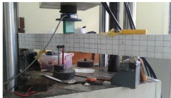
Fig. 6 Three-point bending test for RC beam
