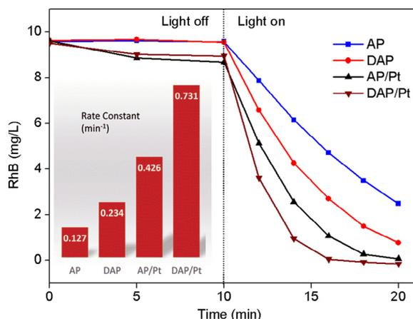
**Fig. 4.** Photocatalytic activity of  $\text{Ag}_3\text{PO}_4$  (AP), defect- $\text{Ag}_3\text{PO}_4$  (DAP),  $\text{Ag}_3\text{PO}_4/\text{PtCl}_6^{2-}$  (AP/Pt), and defect- $\text{Ag}_3\text{PO}_4/\text{PtCl}_6^{2-}$  (DAP/Pt).
