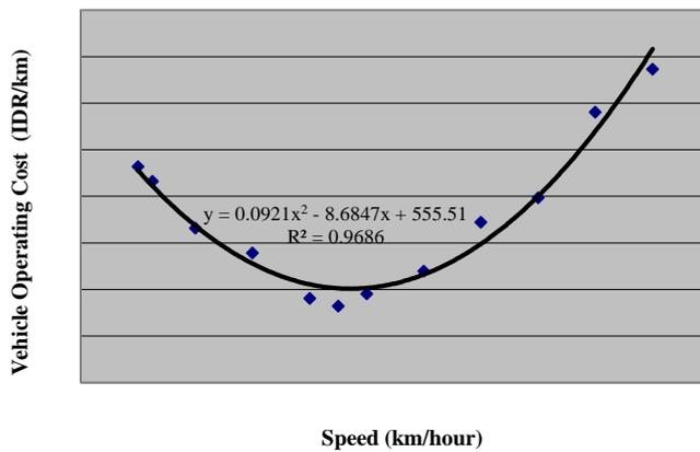
Figure 2 Relationship between speed and vehicle-operating cost [6,14].
