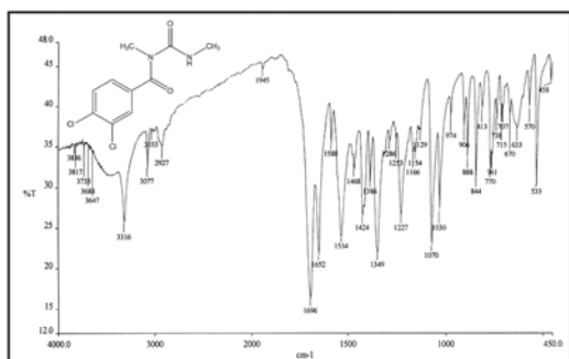
Figure 2. IR spectra of 1-(3,4-dichlorobenzoyl)-1,3-dimethylurea in KBr
