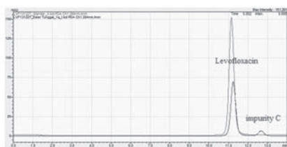
Figure 2. Chromatogram of levofloxacin and impurity C
