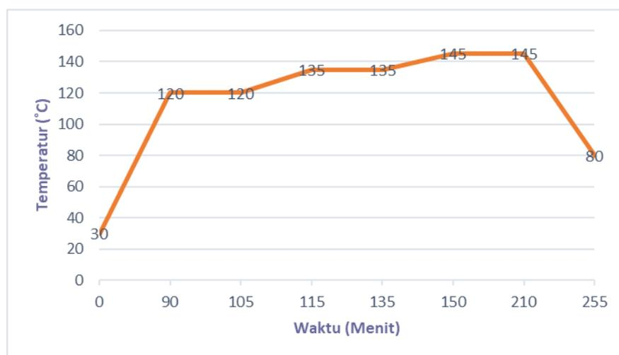
Gambar 2. Program Temperatur Proses Pencelupan Kain<sup>11</sup>
