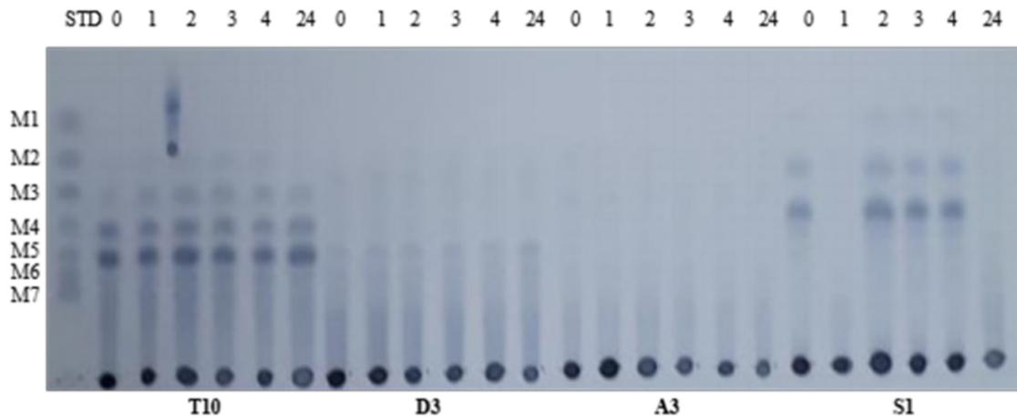
**Figure 6.** The product profile of starch hydrolyzed by amylase of the amylolytic bacteria (T10, D3, A3, and S1) using a TLC method with standards (STD) on times (hours): of 0, 1, 2, 3, 4, and 24 at 30°C. The Standards (STD): monosaccharide (M1), maltose (M2), maltotriose (M3), maltotetraose (M4), maltopentaose (M5), maltohexaose (M6) and maltohepta (M7).
