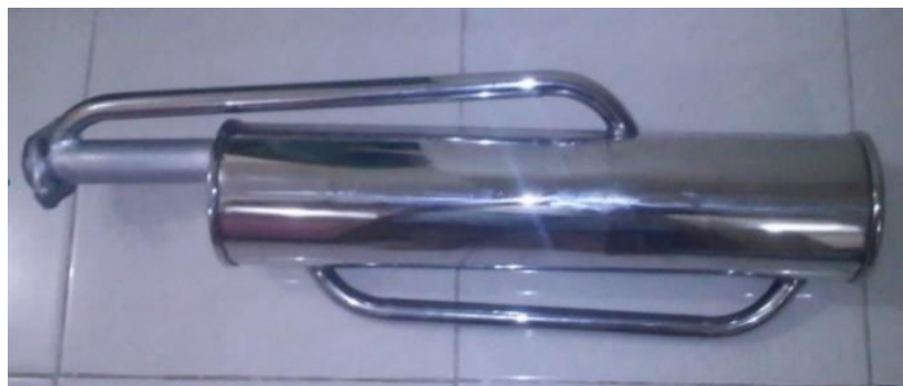
Figure 7. Real form of the muffler with re-heater.
