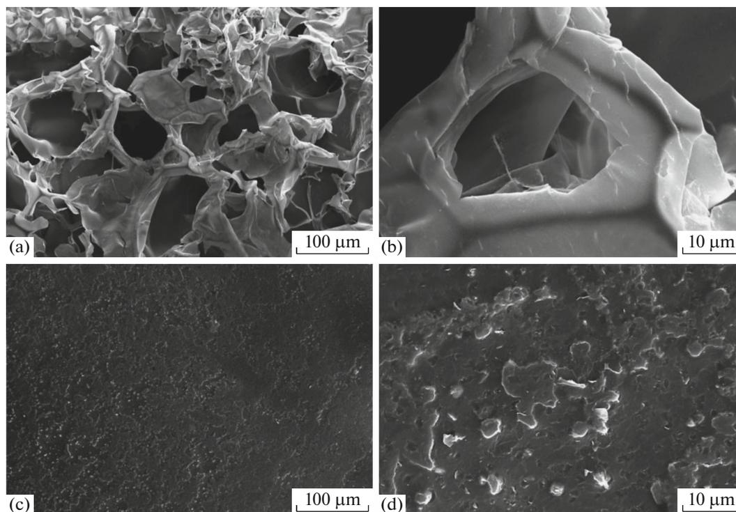
**Fig. 2.** SEM images of chitosan cryogel surface at  $\times 250$  (a) and  $\times 2000$  (b) showed a porous structure. The SEM image of non-cryogel chitosan showed a flat surface at  $\times 250$  (c) and rough surface without pores at  $\times 2000$  (d).
