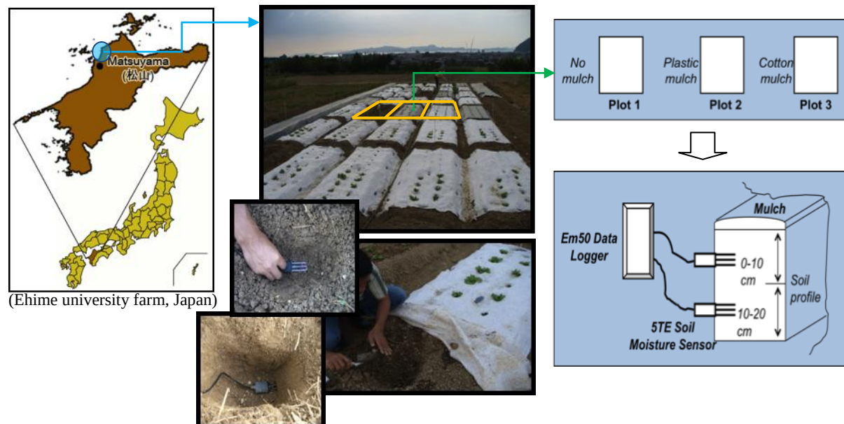
Fig. 1. Schematic diagram of the field monitoring for water content, temperature, and EC in the lettuce growing soil with three different mulches coverage.
