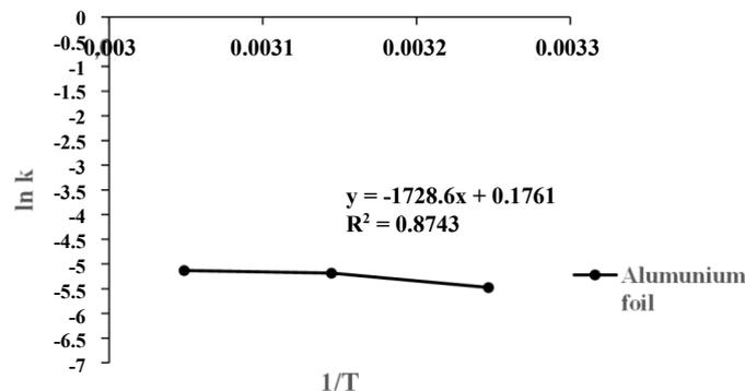
**Figure 2.** The correlation curve between  $\ln k$  and  $1/T$  of the product with aluminum packaging
