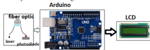
FIGURE 3. Block diagram failure detection system
