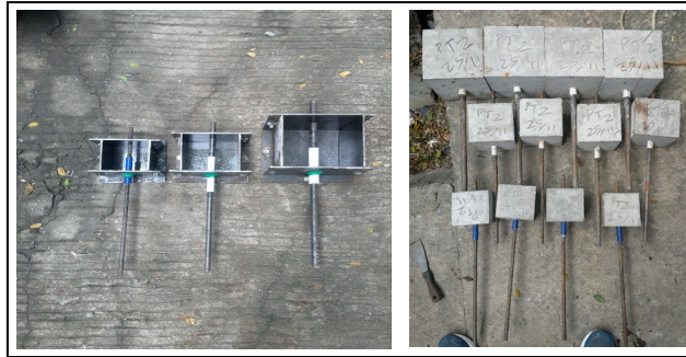
Fig. 2. Moulds and specimens for bond test
