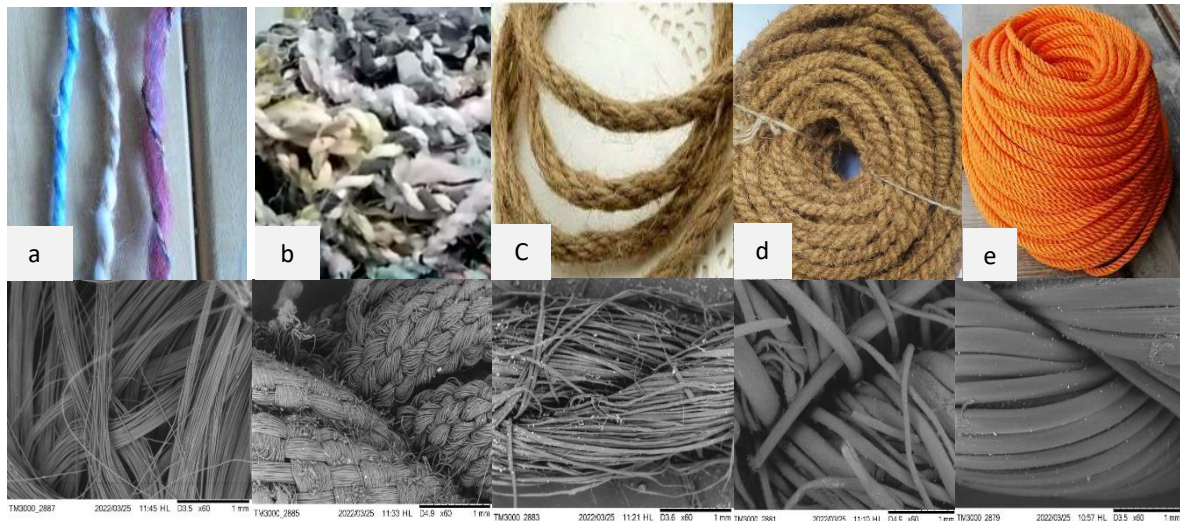
Figure 1. Types of substrates in the experiment took in actual visual (top) and SEM (bottom) with 300x magnifications, a. Rayon ropes (RY), b. Ex-garment rope (CR), c. Brown linen rope (BL), d. Coconut coir rope(CC), and d. Nylon rope(NR).
