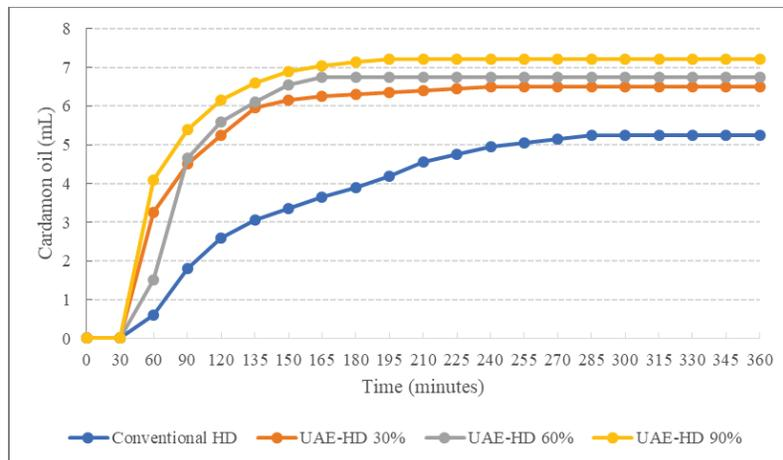
**FIGURE 3.** The relationship of time process hydrodistillation and volume of cardamom oil with various amplitude of ultrasonic compared to conventional technique.
