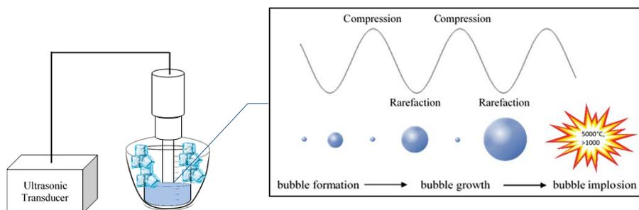
**FIGURE 1.** Cavitation Mechanism in Ultrasonic Pre-treatment [9].
