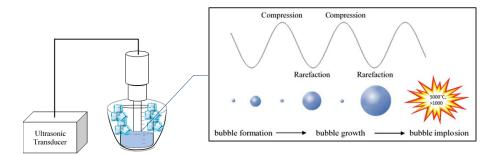
FIGURE 1. Cavitation Mechanism in Ultrasonic Pre-treatment [9].
